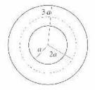
Apply Ampere's law to a circular path of radius 2*a*.  $B(2\pi r) = \mu_0 I_{encl}$   $I_{encl} = I\left(\frac{(2a)^2 - a^2}{(3a)^2 - a^2}\right) = 3I/8$
